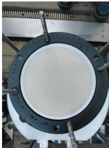
A Glass Fiber Filter used to collect particulate organic matter (POM), i.e. solid debris of marine life often known as "marine snow", from seawater samples. JAMSTEC©
